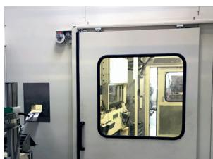
More and more machines are equipped with sound-proof enclosures to reduce the level of noise. Access to the machine usually takes place through sliding doors in the enclosure. In order for the machine to operate, the access doors must always be securely closed and a safety contact established.
