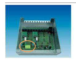
To establish the global emergency-open function (when pressing the emergency-open switch on one door all doors of the interlock system are released) you have to retrofit the pluggable additional relay, part no. 710953. It is simply plugged in the provided socket (see below!). Besides that you have to remove on all control boards of the central controller RJ the jumper JP1 (respectively plug in on one pin only).
