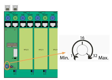
Adjust the time with the potentiometer R1 to the shortest period (minutes).
