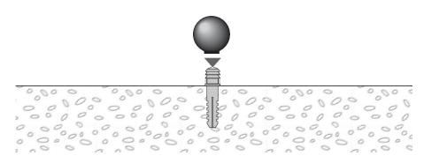
Fix the final stop on the floor as a mechanical stop when opening.
