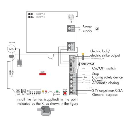
The illustration shows the most important connections of the EL 38 electronic control unit.
