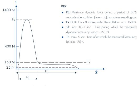
Maximum dynamic force (**Fd**) allowed between both closing edges: Opening width 50 - 500 mm > 500 mm 400 N 1400 N
