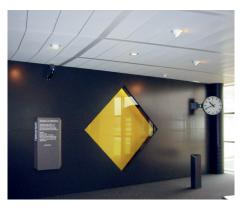
Two very large sliding leaves run on two parallel rails. The closing edges are cut out in such a way that, when they are open, a square standing on one corner reveals the entire yellow background.
