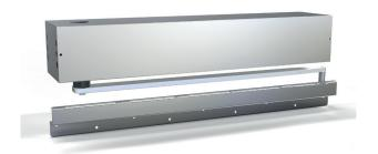
The operator IS equipped with a mechanical braking device which guarantees the required stopping distances under all conditions. The built-in thermal sensor protects the drive from inadmissible loads. Position detection by means of built-in encoder is standard and allows extremely accurate positioning.
