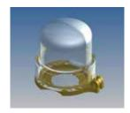
In case the emergency-open switches in an interlock control system are again and again misused, they can be protected by a cover that is prepared for a lead seal (part no. 710839). This cover can be retrofitted and is from transparent, UV resistant plastics with a yellow collar for fixing.
