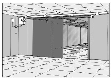
The operator hold-open system is connected to the power pack and the smoke detectors so that its 24 VDC power supply is interrupted in the event of an alarm.
