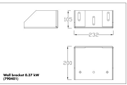
Use of the wall bracket 0.37 kW: - DICTAMAT 900-21, 0.37 kW door operator
