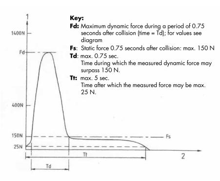
Maximum dynamic force (Fd) allowed between both closing edges:Opening width50 - 500 mm400 N1400 N
