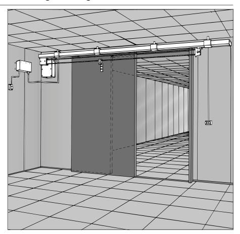
DC door operators with integrated encoder
