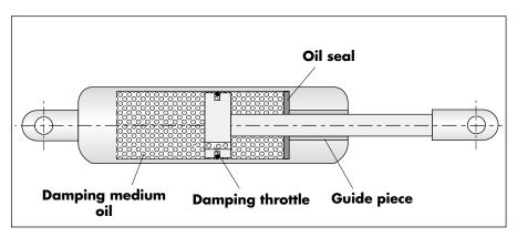
The **adjustable oil dampers with fixings on both ends (ÖDR)** use the stepped adjustment of the final dampers. The damping is adjusted by pulling and turning the piston rod.
