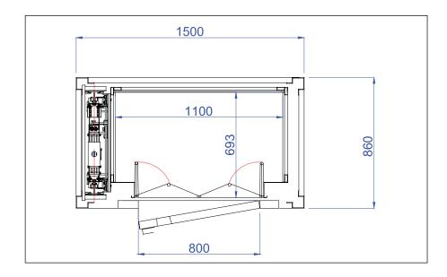
Homelift DHM 500 in an Extremely Narrow Stair Well with Glass Cabin Walls Despite the extremely little depth of this stair well (860 mm!) the customer wanted a cabin with glass walls. As a shaft was used the DICTATOR lift shaft system with glass panels to keep the staircase as "open" and bright as possible.
