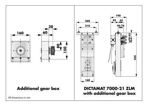
The DICTATOR additional gear box is put on top of the basic module of the door operator and fixed with two lateral connection plates. The driving wheel of the operator is taken off and the small chain wheel placed there instead. This chain wheel is connected by a chain with the chain wheel on the additional gear box. Afterwards the cover is remounted.
