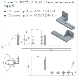
When selecting this bracket, please note that the specified DIN direction applies to installation on push side.
