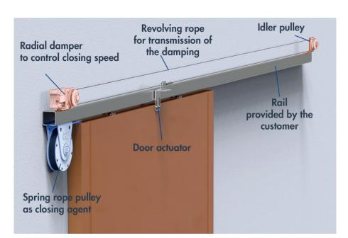
The components of the DICTA-MAT 50 BK can be combined at will. For the most common applications standard kits have been prepared. When they cannot be used, the components can be combined individually. Depending on the available space, the components of the modular system can be mounted in different positions. For designers there are nearly no limits to develop own object specific solutions. Of course, DICTATOR will be happy to assist you in realizing your ideas.
