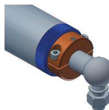
**Adjustment lock for DIREKT with ball and socket joints (for ascending hinges):** Here it is not possible to simply slip the adjustment lock on top of the wheel. Therefore this adjustment lock consists of two parts, which can be clipped on from both sides, screwed together and secured with an extra screw.
