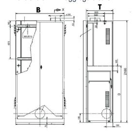
The DICTATOR DHE lift does not require a separate machine room. Instead, hydraulic power unit and control system are housed in an approved caret. There are two different sizes available, depending on the particular model. Dimensions (width x depth x height)
